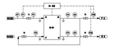
(The input water is the output of two-stages Reverse Osmosis Plant)
