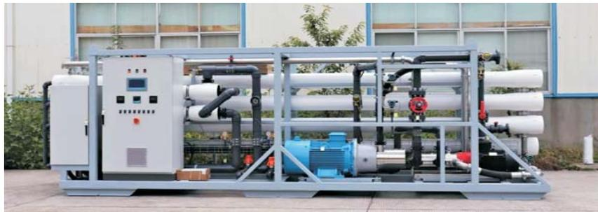
High Purity Water Systems—Electrodeionization System (EDI System) Treatment Process
