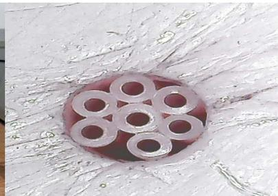
Microscope of Hollow Fibers
